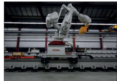
TMF-5 traversing axis with ABB robot
